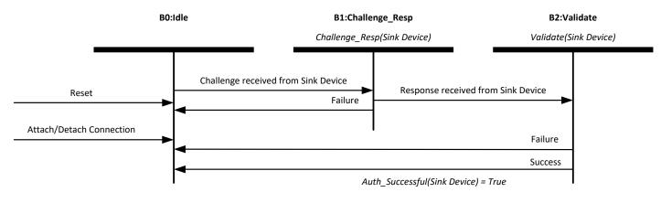
The following figure shows the *Auth(Device)* state machine from the point of view of a **sink device** receiving an Authentication request from a source device. The detail of this state machine including the function to calculate  $K'_{AUTH}$  is described in the DTCP2 Specification available under license from the DTLA.
